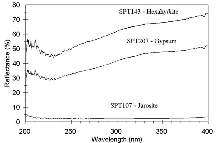
Fig. 9. Reflectance spectra (200–400 nm) of sulfate minerals (<45  $\mu\text{m}$ ). Sample compositions are provided in Table 1.
