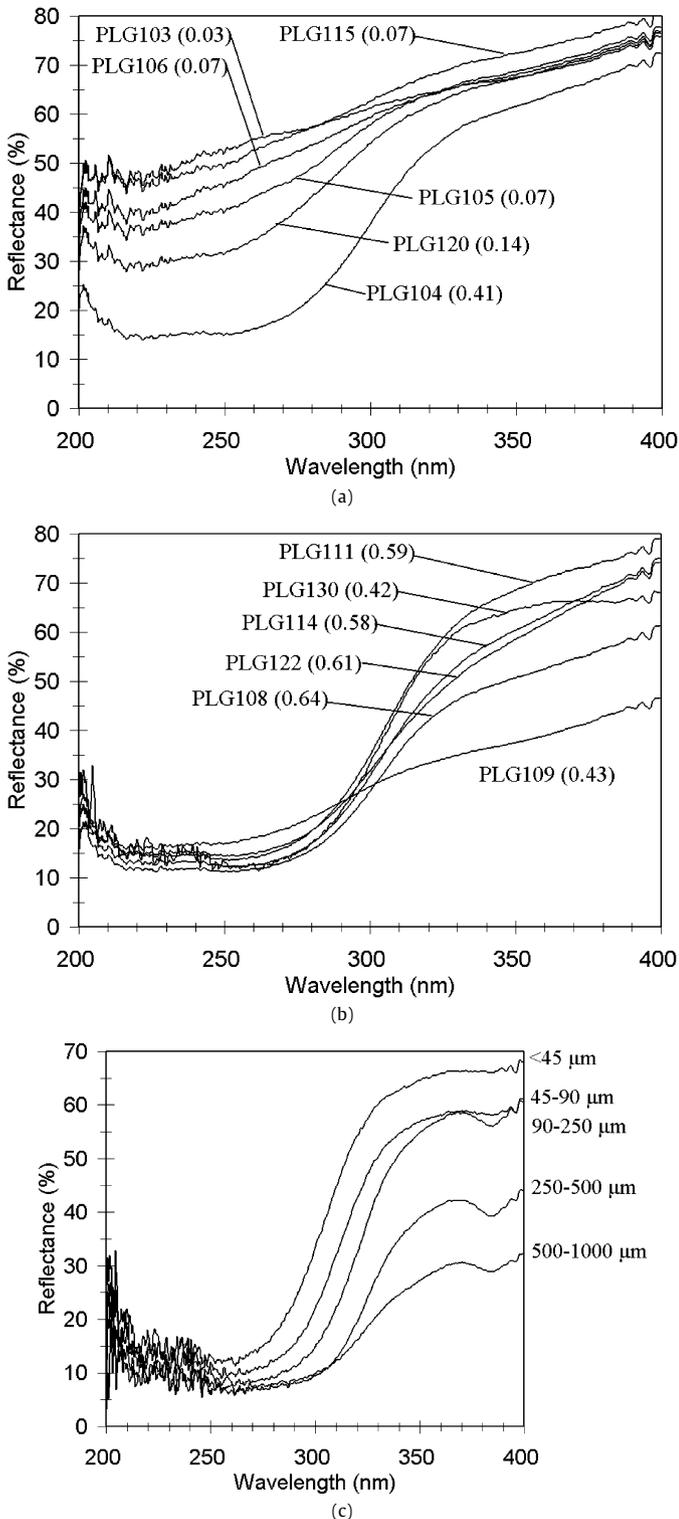
**Fig. 6.** Reflectance spectra (200–400 nm) of plagioclase feldspars: (a) for the lower Fe-content members (<45  $\mu\text{m}$ ); (b) for the higher Fe-content members (<45  $\mu\text{m}$ ); (c) PLG130 reflectance spectra as a function of grain size, Fe content (as wt%  $\text{Fe}_2\text{O}_3$ ) is indicated for each sample. Sample compositions are provided in Table 1.
