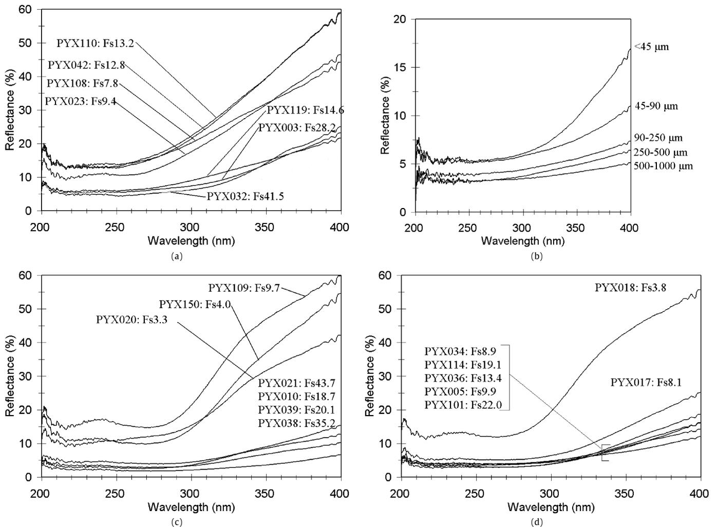
**Fig. 5.** Reflectance spectra (200–400 nm) of pyroxenes: (a) low-calcium pyroxenes (<45  $\mu\text{m}$ ); (b) low-calcium pyroxene PYX032 for various grain sizes; (c) spectral type A high-calcium pyroxenes (<45  $\mu\text{m}$ ); (d) spectral type B high-calcium pyroxenes (<45  $\mu\text{m}$ ). Sample compositions are provided in Table 1. Ferrosilite contents (mol% Fs) are indicated for each sample in (a), (c), and (d).
