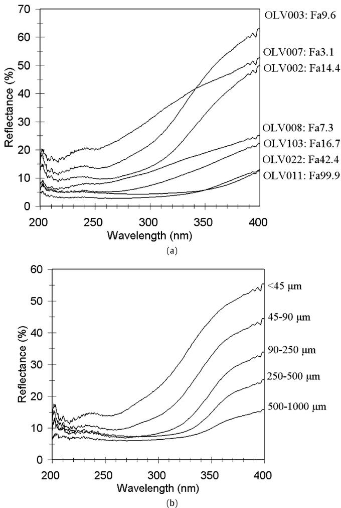
**Fig. 4.** Reflectance spectra (200–400 nm) of olivines: (a) as a function of composition (all <45 μm); and (b) OLV003 as a function of grain size. Sample compositions are provided in Table 1.
