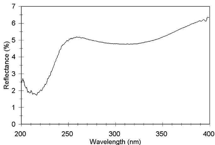
Fig. 1. Reflectance spectrum of BaSO<sub>4</sub> relative to UV mirror used to correct spectra for deviations from ideal reflectance for BaSO<sub>4</sub>.
