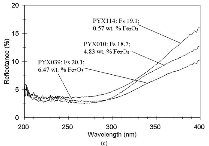
**Fig. 11.** Reflectance spectra of three different sets of high-calcium pyroxenes: (a) two samples with similar  $\text{Fe}^{2+}$  but different  $\text{Fe}^{3+}$  contents: PYX005 and 009; (b) four samples with no apparent  $\text{Fe}^{3+}$  from wet chemical analyses (PYX009, 018, 020, and 150); and (c) three samples with similar  $\text{Fe}^{2+}$  but different  $\text{Fe}^{3+}$  contents (PYX010, 039, 114).
