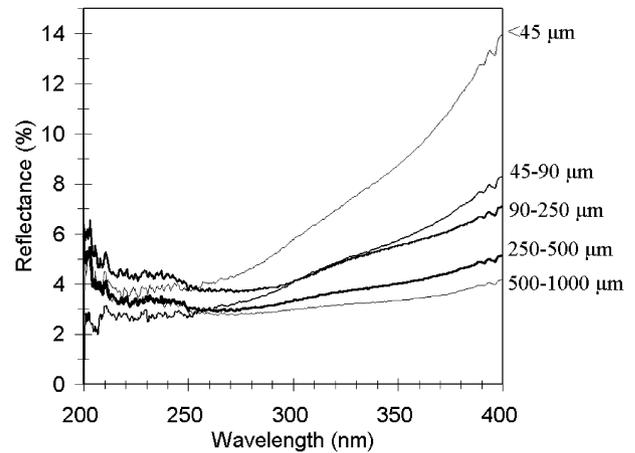
**Fig. 7.** Reflectance spectra (200–400 nm) of basalt SA-51 for different grain sizes. Sample composition is provided in Table 1.
