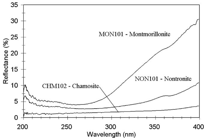
Fig. 8. Reflectance spectra (200–400 nm) of phyllosilicates (<45  $\mu\text{m}$ ). Sample compositions are provided in Table 1.
