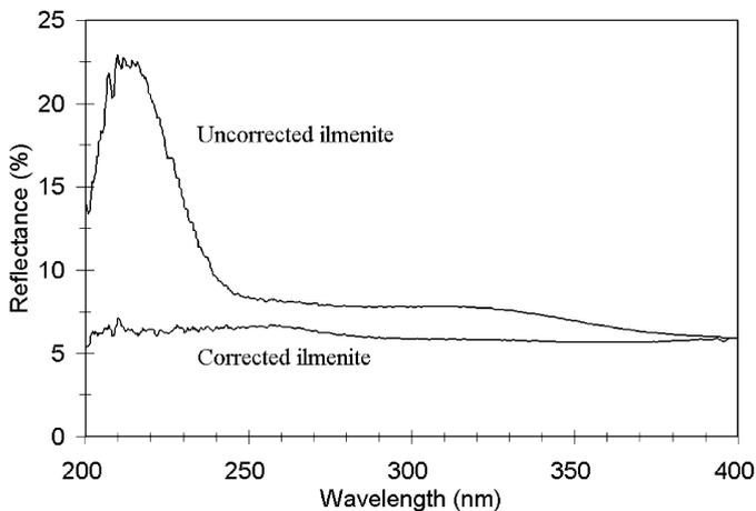
Fig. 2. Reflectance spectrum of ilmenite (ILM101, <45 μm) measured against BaSO<sub>4</sub> and corrected for deviations of BaSO<sub>4</sub> reflectance from ideality.
