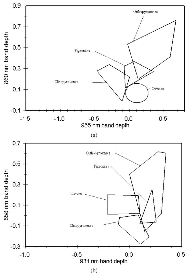
Fig. 9. 955 nm versus 860 nm (a) and 931 nm versus 858 nm (b) band depths for various mafic silicates. See text for description of band depth calculations.
