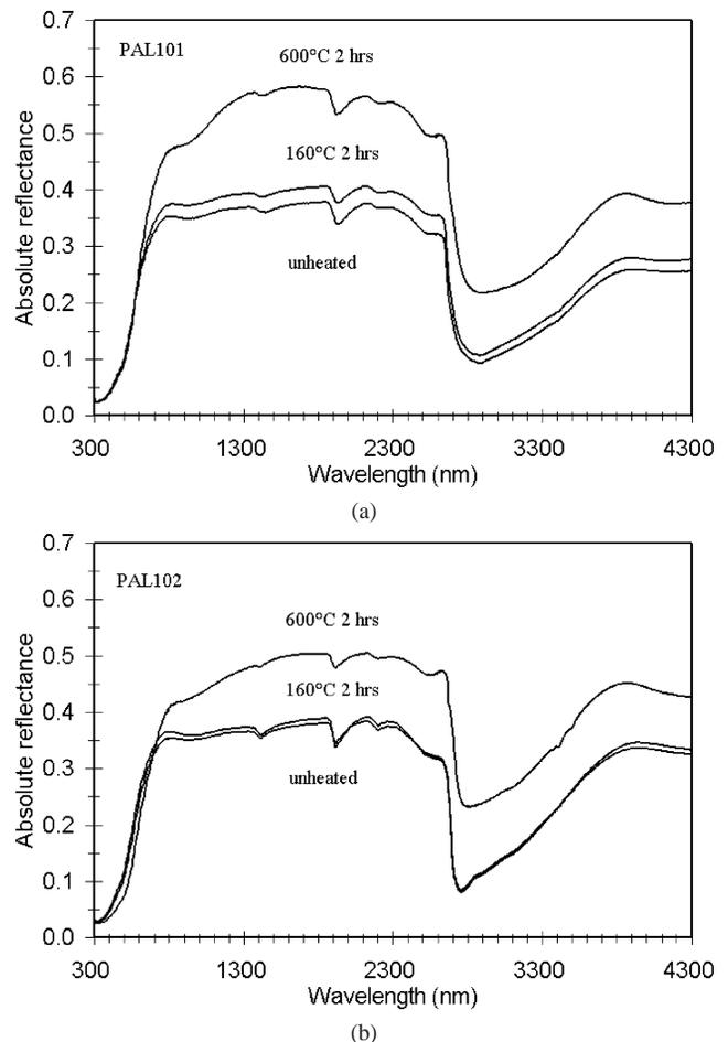
Fig. 1. 300–4300 nm reflectance spectra of palagonitic material samples PAL101 (a) and PAL102 (b), unheated and heated in air to 160 and 600 °C for 2 hours. See Table 1 for compositional information.
