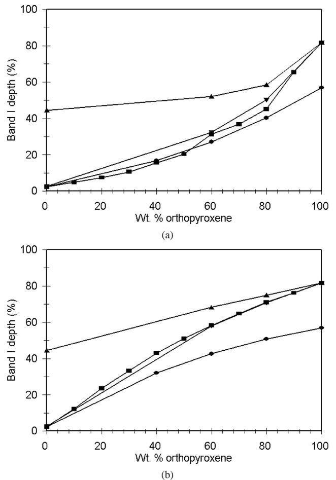
Fig. 4. Variations in depth of the Band I feature in the intimate (a) and areal (b) mixtures of orthopyroxene (PYX110) and palagonitic material (PAL101, PAL102) or hematite (HEM101). Symbols are the same as those in Fig. 3. Interpolating values between points separated by more than 20 wt% orthopyroxene may not be valid.
