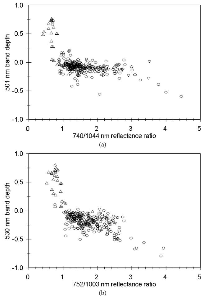
Fig. 12. 501 nm band depth versus 740/1044 nm (a) and 530 nm band depth versus 752/1003 nm (b) reflectance ratios for hematite ( $\Delta$ ), and mafic silicates and martian meteorites ( $\circ$ ).
